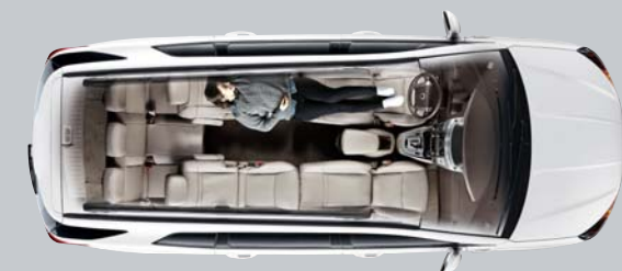
Front and 2nd-row seats flat (converts into beds for driver and front passenger)
