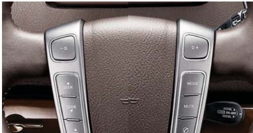
Audio remote control on steering wheel
